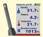
measurement of relative humidity, temperature and barometric pressure
