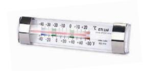
This spirit-filled fridge/freezer thermometer is encased in a clear ABS housing (20 x 30 x 122 mm). The thermometer's colour-coded zones indicate temperature over the range of -40 to 20 °C and -40 to 80 °F with a 1 °C resolution.
